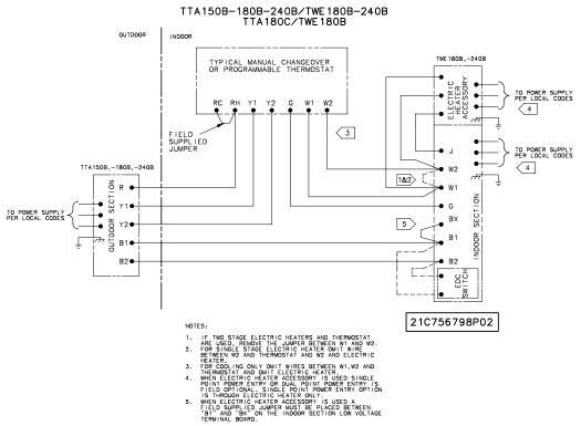
Figure 22. TTA150B, 180B, 240B/TWE180B, 240B; TTA125B, 155B, 200B/TWE155B, 200B; TTA155C/TWE155B; TTA180C/TWE180B
